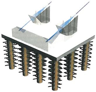
The large anchor being considered for use in the bridge in Ma'anshan, China, includes 18 rooted caissons arranged in seven rows. A bearing platform measuring 71 by 59 m tops the caissons.
